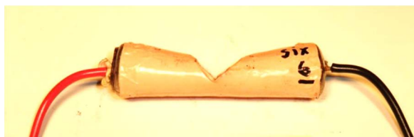
Fig. 8. Photograph showing an LG Chem cell crushed by the plastic wedge that did not rupture nor ignite 6.5% CH 4 -air at 40 °C ambient temperature. The cell hard shorted.
